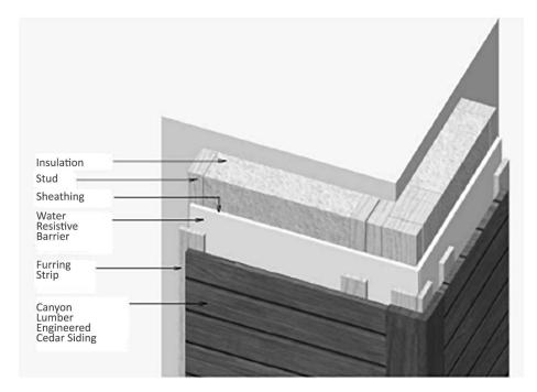
3) <u>Corner boards installed over siding/panelling:</u> Do not apply caulk or sealant at the joint between the corner boards and the Product, with this installation method.
