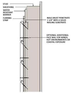
FASTENERS MUST PROVIDE 1 1/2" PENETRATION INTO A SOLID, NAILABLE SUBSTRATE (INTO STUDS OR A COMBINATION OF FURRING STRIPS, SHEATHING AND/OR STUDS)
