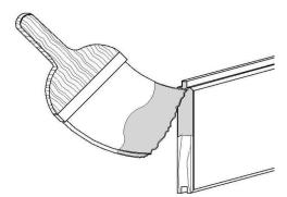
\*\*ALL END GRAIN AND JOB-SITE CUTS MUST BE COATED TO PREVENT WATER ABSORPTION!\*\*
