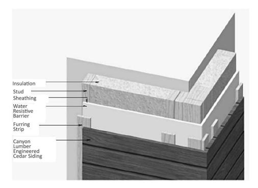
2) Siding/Panelling installed next to corner boards: Leave a 1/8" gap between the Product and corner boards to allow for a properly applied bead of caulking or sealant between the two materials. Follow caulking or sealant manufacturer's instructions.
